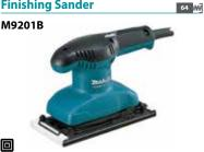
Continuous rating input 180W Pad Size 93 x 185 mm (3-5/8" x 7-1/4") Abrasive Paper Size 93 x 228 Orbits Per Minute (OPM) 12,000 Sanding Metal Plate: 6 m/s<sup>2</sup> 74 dB(A) 214x92x147 mm Vibration Level Sound Pressure Level  $(I \times W \times H)$ (8-3/8"x3-5/8"x5-3/4") Power supply cord
