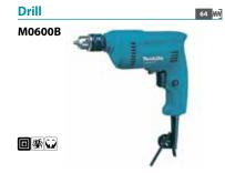
Continuous rating input 350W Steel: 10 mm (3/8", Capacity Wood: 20 mm (13/16") No Load Speed (RPM) 0 - 3,000 Vibration Level Drilling Into Metal: 3.0 m/s<sup>2</sup> Sound Pressure Level 77 dB(A) 230x66x176 mm (9"x2-5/8"x6-15/16") (LxWxH)Net weight 1.2 kg (2.6 lbs) Power supply cord
