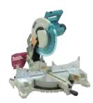
Continuous rating Input 1,650W 305 mm (12") Blade Diameter 25.4, 30 mm (1, 1-3/16") 48 / 48° L 48, 48° R Hole Diameter Bevel Angle 45° L Max Cutting Capacity 0°: 98 x 153 mm (3-7/8 x 6" 45°: 70 x 149 mm (2-3/4 x 5-7/8") No Load Speed (RPM) 674 x 610 x 607 mm (26-1/2 x 24 x 23-7/8") Dimensions (L x W x H)
