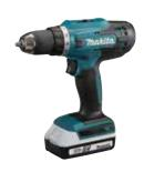
Capacity Chuck Capacity No Load Speed (RPM) Steel / Wood: 13 / 36 mm (1/2 / 1-7/16") 1.5 - 13 mm (1/16 - 1/2") High / Low: 0 - 1,400 / 0 - 400 Max Fastening Torque Hard / Soft: 42 / 24 N·m (370 / 210 in.lbs.) Dimensions (L x W x H) w/BL1815G: 221 x 83 x 240 mm (8-3/4 x 3-1/4 x 9-1/2") 1.7 kg (3.7 lbs.) Net weight
