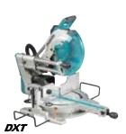
Continuous rating Input 1.800W Blade Diameter 305 mm (12") 48 / 48° L 48, 48° R 60 / 60° L 60, 60° R Bevel Angle Miter Angle Max Cutting Capacity 0°: 92, 107 x 363, 382 mm (3-5/8, 4-1/4 x 14-1/4, 15") 45°: 92, 107 x 255, 268 mm (3-5/8, 4-1/4 x 10, 10-1/2") No Load Speed (RPM) 3,200 898 x 664 x 725 mm Dimensions (L x W x H) (35-1/4 x 26-1/8 x 28-1/2") 29.5 kg (65 lbs.) 2.5 m (8.2 ft) Net weight Power supply cord
