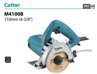
Continuous rating input 1,200W Blade Diameter Max Cutting Capacity 110 mm (4-3/8" No Load Speed (RPM) 13,000 Concrete Cutting: 5.5 m/s<sup>2</sup> Vibration Level Sound Pressure Level Sound Power Level 100 dB(A) 111 dB(A) Dimensions 227x209x166 mm (LxWxH)(8-15/16"x8-1/4"x6-1/2") 2.9 kg (6.4 lbs) 2.0 m (6.6 ft.) Net weight Power supply cord
