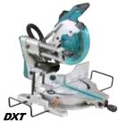
Continuous rating Input 1.510W Blade Diameter 260 mm (10-1/4") 48 / 48° L 48, 48° R 60 / 60° L 60, 60° R Bevel Angle Miter Angle Max Cutting Capacity 0°: 68, 91 x 279, 310 mm 45°: 68, 91 x 197, 218 mm No Load Speed (RPM) 3,200 Dimensions (L x W x H) 805 x 644 x 660 mm (31-3/4 x 25-3/8 x 26" Net weight 26.3 kg (57.9 lbs.) Power supply cord 2.5 m (8.2 ft)
