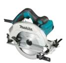
Continuous rating Input 1,600W 185 / 190 mm (7-1/4 / 7-1/2") 15.88, 20, 30 mm (5/8, 13/16, 1-3/16") 0°: 65, 67 mm (2-9/16, 2-5/8") 45°: 44, 45 mm (1-3/4, 1-3/4") Blade Diameter Hole Diameter Max Cutting Capacity No Load Speed (RPM) 5.500 300 x 240 x 261 mm (11-3/4 x 9-1/2 x 10-1/4") Dimensions (L x W x H) Net weight 4 kg (8.9 lbs.)
